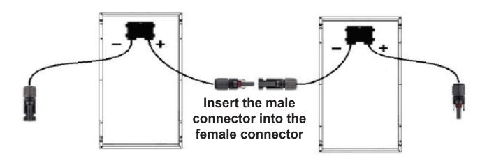
Install and connect the PicoCell™ Panel
